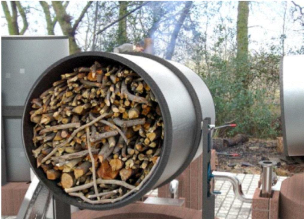
The above horizontal bed unit is designed to be run 24/7, like a manufacturing plant, whereas the batch kiln is designed to be run intermittently. The tilting mechanism allows for easy loading and unloading. It is also possible to configure 3 units in a round robin fashion so that the excess heat from one is used to start the pyrolysis process in another. These units require no electricity, but there is more manual labor involved in preparing the feedstock, loading and unloading the units.
